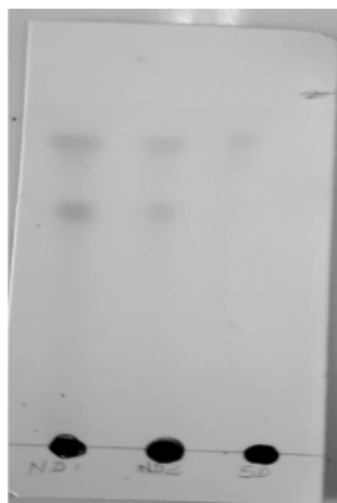
Figure 23 TLC of natural and synthetic indigo dye extract
