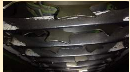
Figure 1 Damaged plucking roller
